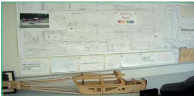
Fuselage prototype for a ¼ scale aircraft being built by the engineering students.
